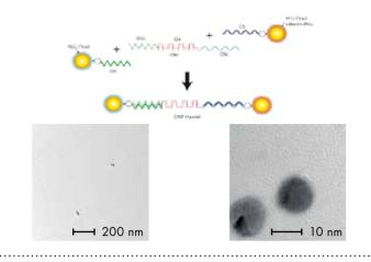
Top: Synthesis strategy for gold nanoparticle dimers seperated by a DNA strand. The dimers are created by binding functionalised gold nanoparticles to the sticky ends of a DNA strand. Bottom: Electron microscopy images of the synthesised gold nanoparticle pairs, which have been separated from monomers and trimers by electrophoresis. The particles are separated by 30 nm.
