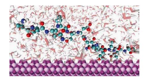
Fully atomistic simulations of a synthetic oligopeptide (AQNPSDNNTATA) at the watersemiconductor interface
