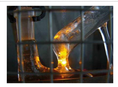
"Burning water" in a high frequency electromagnetic field
