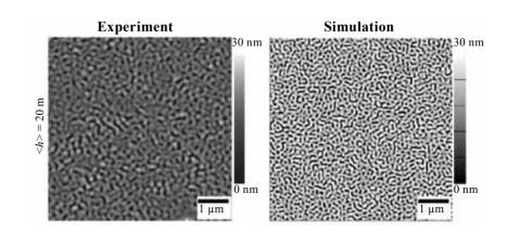
Comparison of experiments (*left*) and computer simulations (*right*) on structure formation during vapor deposition of thin polycarbonate films on GaAs
