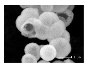
Zirconia hollow spheres with mesoporous walls as supports for metal catalysts in high-temperature conversions
