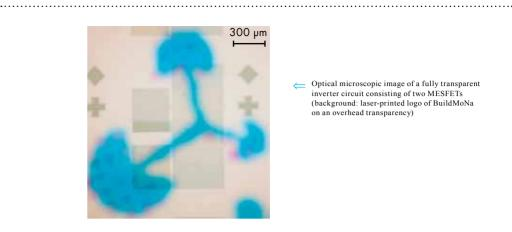
Optical microscopic image of a fully transparent inverter circuit consisting of two MESFETs (background: laser-printed logo of BuildMoNa on an overhead transparency)
