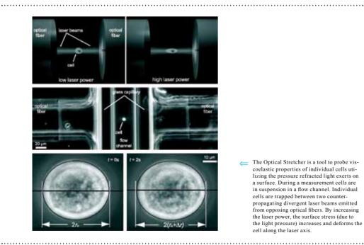
The Optical Stretcher is a tool to probe viscoelastic properties of individual cells utilizing the pressure refracted light exerts on a surface. During a measurement cells are in suspension in a flow channel. Individual cells are trapped between two counterpropagating divergent laser beams emitted from opposing optical fibers. By increasing the laser power, the surface stress (due to the light pressure) increases and deforms the cell along the laser axis
