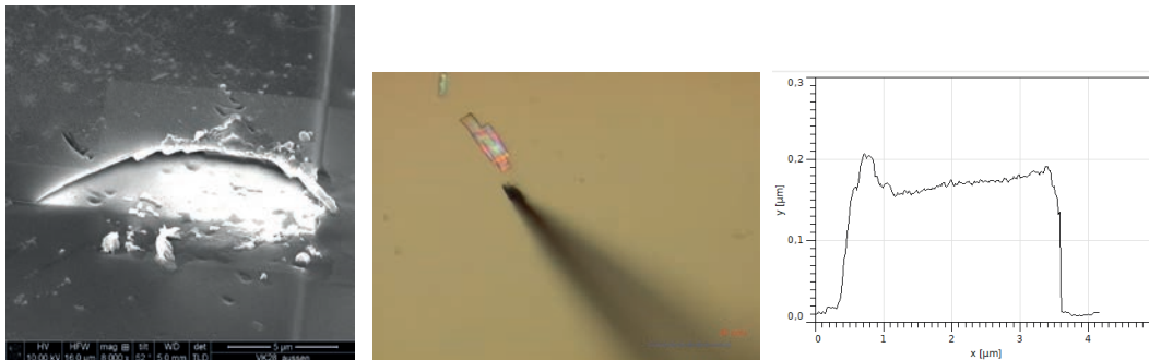
↑ Fig. 2. (a) SEM side view of a diamond membrane created by 30 keV H implantation, (b) diamond layers with a thickness of 180nm. (c) AFM image of the diamond layer. The roughness is below 3 nm (C. Scheuner et al. pub. in preparation).
